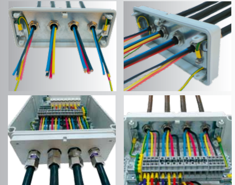
Cable entry for armoured cables via metal glands with earthing
